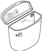
The toilet tank number is imprinted on the inside back of the tank.
